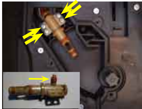
Loosen the four screws indicated and remove the heater valve asm. When refitting it, be careful with the two oil-rings shown in the smaller picture.
