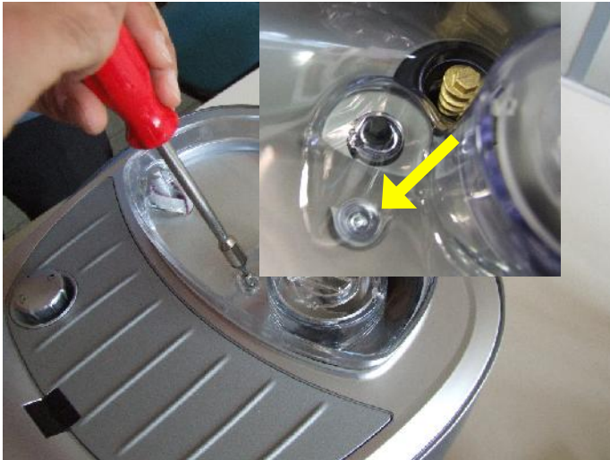
Loosen the screw on the coffee container.
