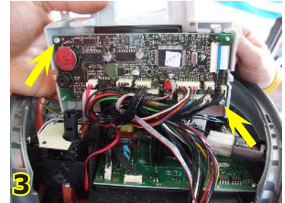
Fig.1 Loosen the screws as indicated and turn the front piece upwards to get to the card.
