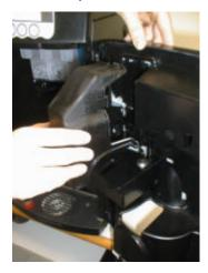
3. Remove the coin-mec protection inside the door;
