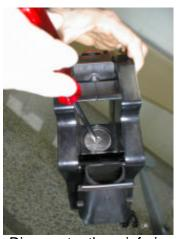
Dismount the inferior filter and clean it with hot water removing all coffee powder.
