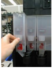
Remove all the ingredients canisters from the machine and disassemble
