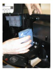
4. Fit the coin-mechanism;
