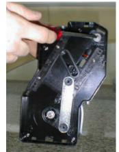
Remove the plates of the superior filter
