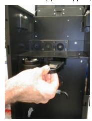
and the aspiration drawers. Immerse all parts in the solution. Using a cloth soaked in the solution, proceed to clean also the attachment bases of the mixers, which remain fixed to the machine. The time
