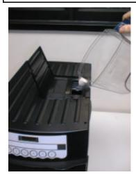
Fill the internal independent water tank using drinking water. If it is necessary demand a laboratory certification to a specific analysis laboratory. To fill in water, lift the water refilling cover or extract the tank from the machine and pour drinking water inside the tank. The capacity of this tank is about 2 litres.
