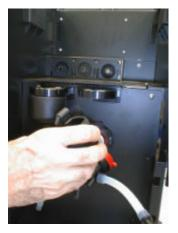
remove the pipes support, remove the mixing bowls, the mixing fan.
