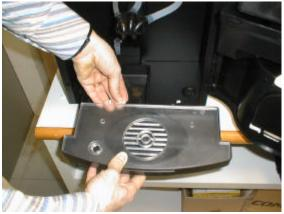
Remove the liquid waste bucket,
